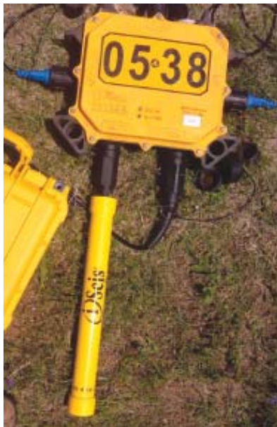
External Wi-fi for long range pass-by harvesting. Passive acquisition operation
