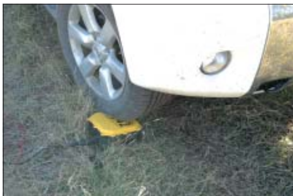
Cableless line boxes must be tough to protect data and prevent tipping
