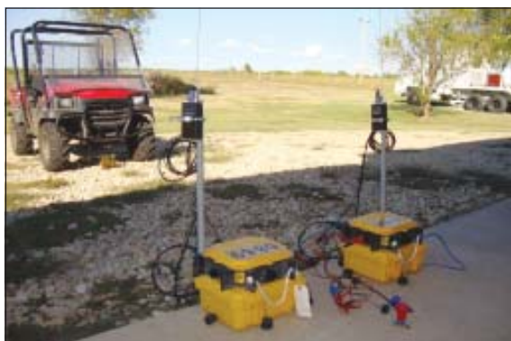
Choices in time stamping. More accurate clocks and VHF timing option for when GPS signals are unavailable
