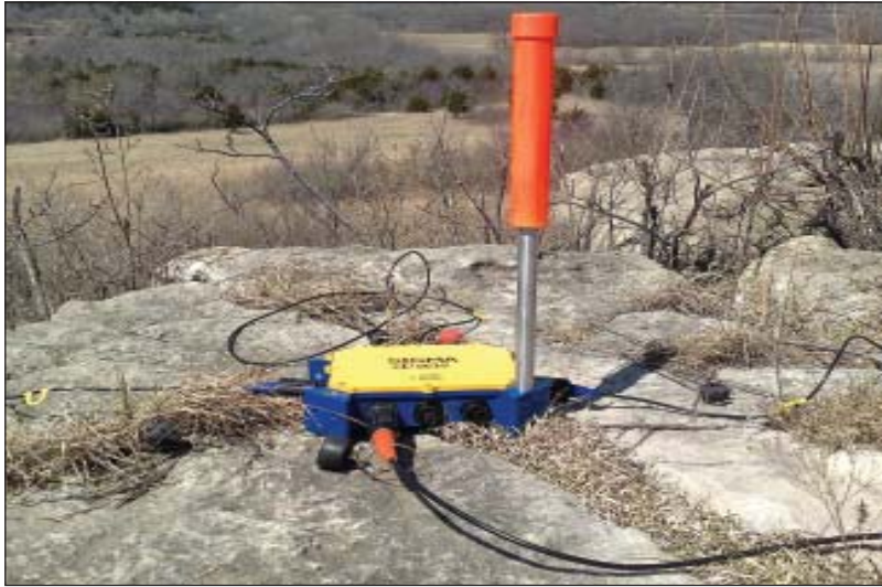
Sigma with optional MRN repeater to increase range
