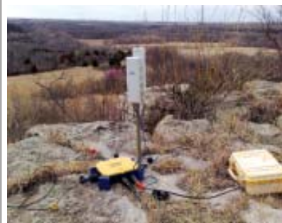
Real-time cableless data transfer using 2.4 GHz semidirectional Wi-fi in daisy chain mode
