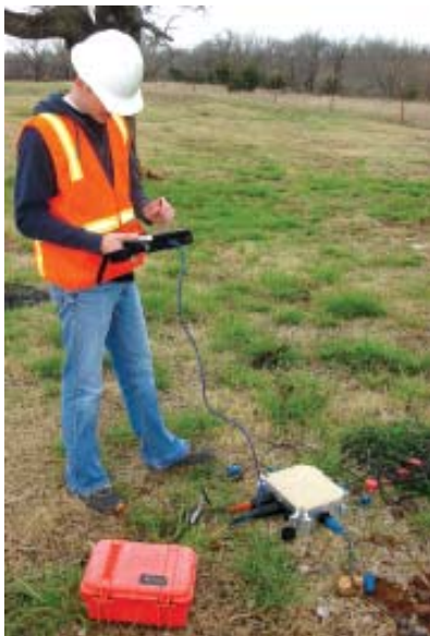
SMART harvesting using Ethernet cable link between PC and line unit, while not interrupting acquisition
