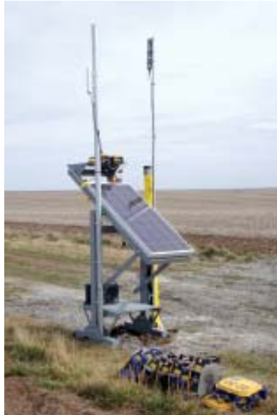
Permanent array (> 2 years, 24/7) using Sigma for real-time data transfer over 750 sq.km area and local storage, USA
