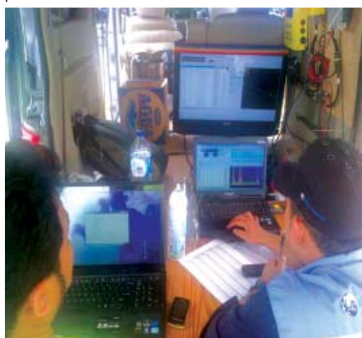
Sigma central system in jungle environment, observer sees real time status of all equipment, essential for best quality data in passive operations.
