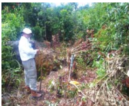
Sigma system showing Mesh Radio repeater in thick jungle. Note: no line of sight exists to neighbouring ground units which in passive operations can be significant distances away, demonstrating the unique ability of the system to operate in such modes.
