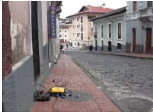
ReMi operation using Sigma system, Old City, Quito, Ecuador. Courtesy iSeis.
