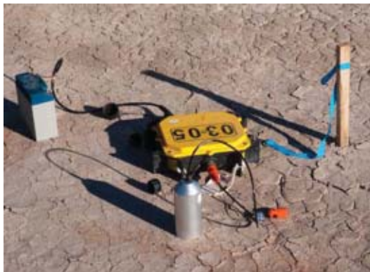
Standard Sigma system using non-standard sensor and low cost (non-lithium) battery. Such flexibility makes multiple operation types possible.
