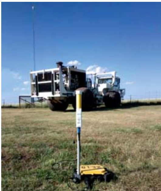
Sigma hyMesh option. Simply plugs into Sigma ethernet port to provide mesh topology ultra high bandwidth for realtime data (10 - 20,000 channels capacity claimed) even in tough environments.
