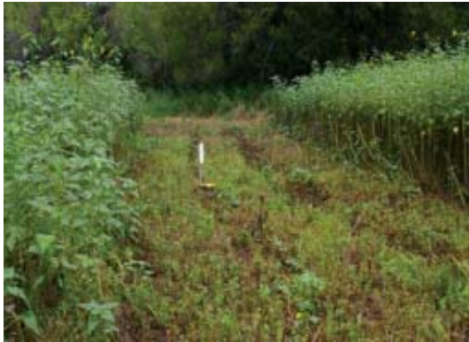
Ongoing testing and characterisation of Sigma system by manufacturer, this time in different cereal plantations. Here showing requirement for directional antenna for long range high bandwidth communications at 2.4 GHz. Omnidirectional antenna in this situation are unreliable due to signal absorption by green vegetation.
