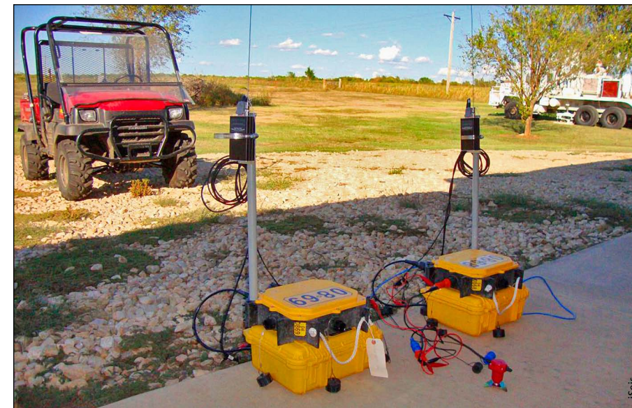
Choices in time-stamping: two Sigma units, which are receiving essential timing information via a VHF synchronisation system, used when GPS signals are unavailable.
