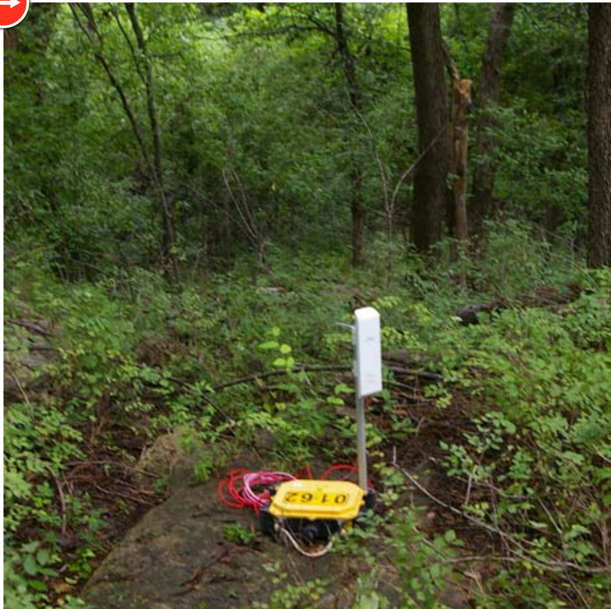
Hilly forested areas present special challenges to all instruments. Flexibility is the key such that a recorder can succeed in any environment with or without another recorder. Sigma with directional WiFi plug-in option.
