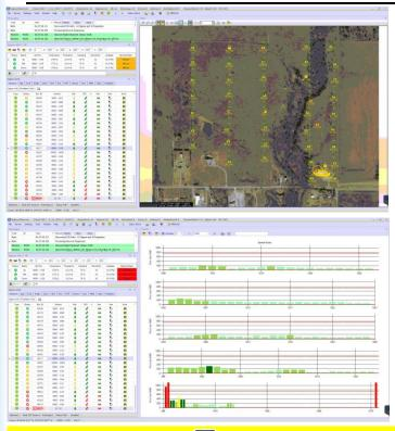
Sigma Observer provides command and control of the Sigma Boxes and enables system monitoring before and during acquisition.
