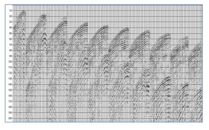
Sigma Harvest reads in the "raw" SEG-Y data files, spatially aligns them according to their deployment, windows the traces in time, and output shot records.
