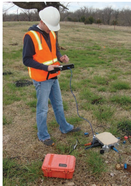
Storing seismic data with no cables using the i-Seis system
