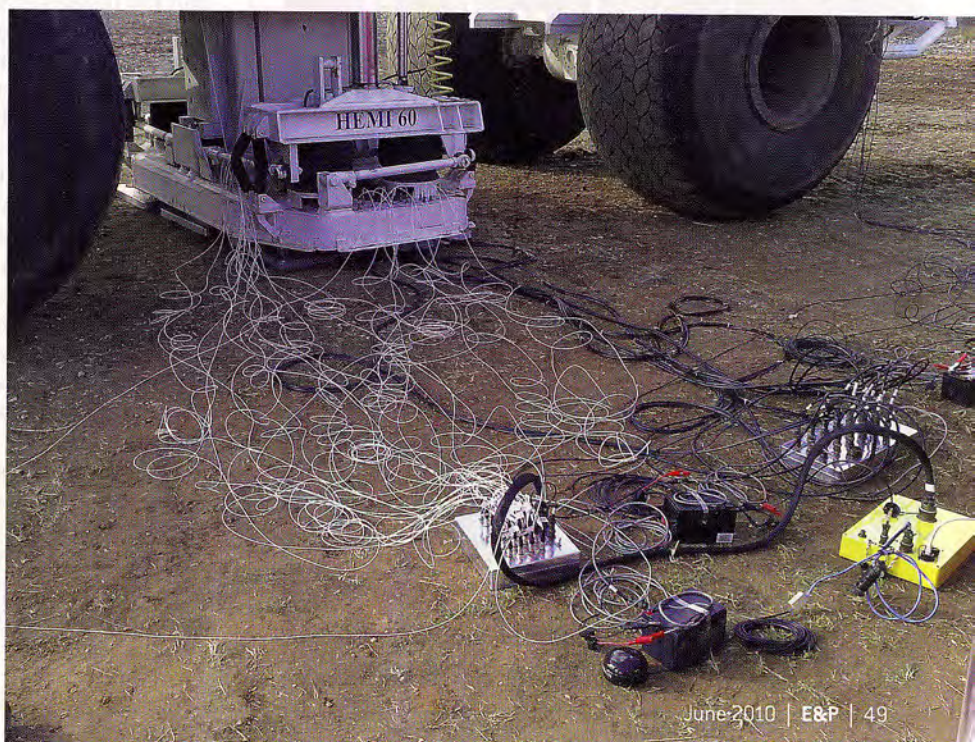
Figure 4. Load cell testing of vibrator performance.
