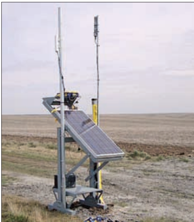
Figure 8 Solar power-assisted cableless acquisition equipment on passive monitoring.
