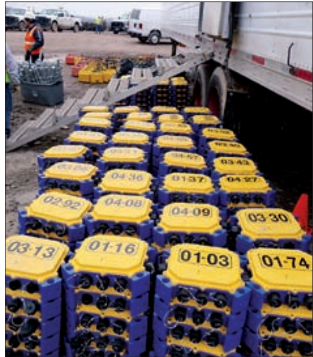
Figure 7 Cableless is increasingly a preferred method of acquisition.
