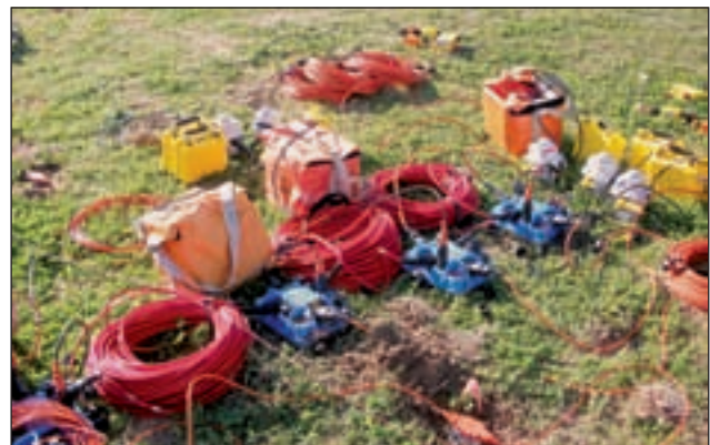
Figure 1 Cabled and cableless systems under test. Relative weights and complexities are apparent.
