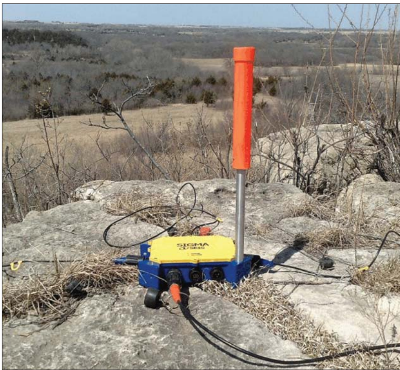
Mesh radio network on iSeis's Sigma system. "Cableless no longer means QC-less."
